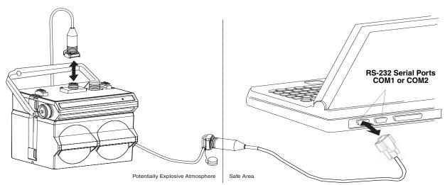
Figure 3-1 Connection to a Laptop, Using Cables P/N 60-2004-336 and 60-2004-339
